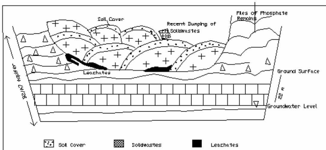
Figure 3. A schematic sketch representing the environmental problems in the closed Rusiefa landfill
