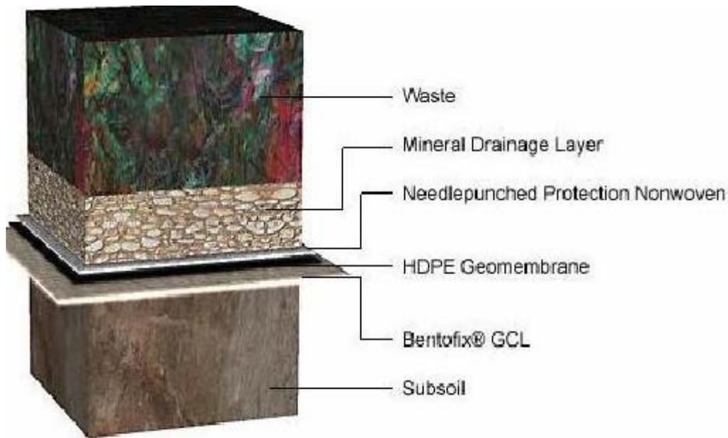
Figure (7): a detailed description of the lineation at Ghabawi landfill
