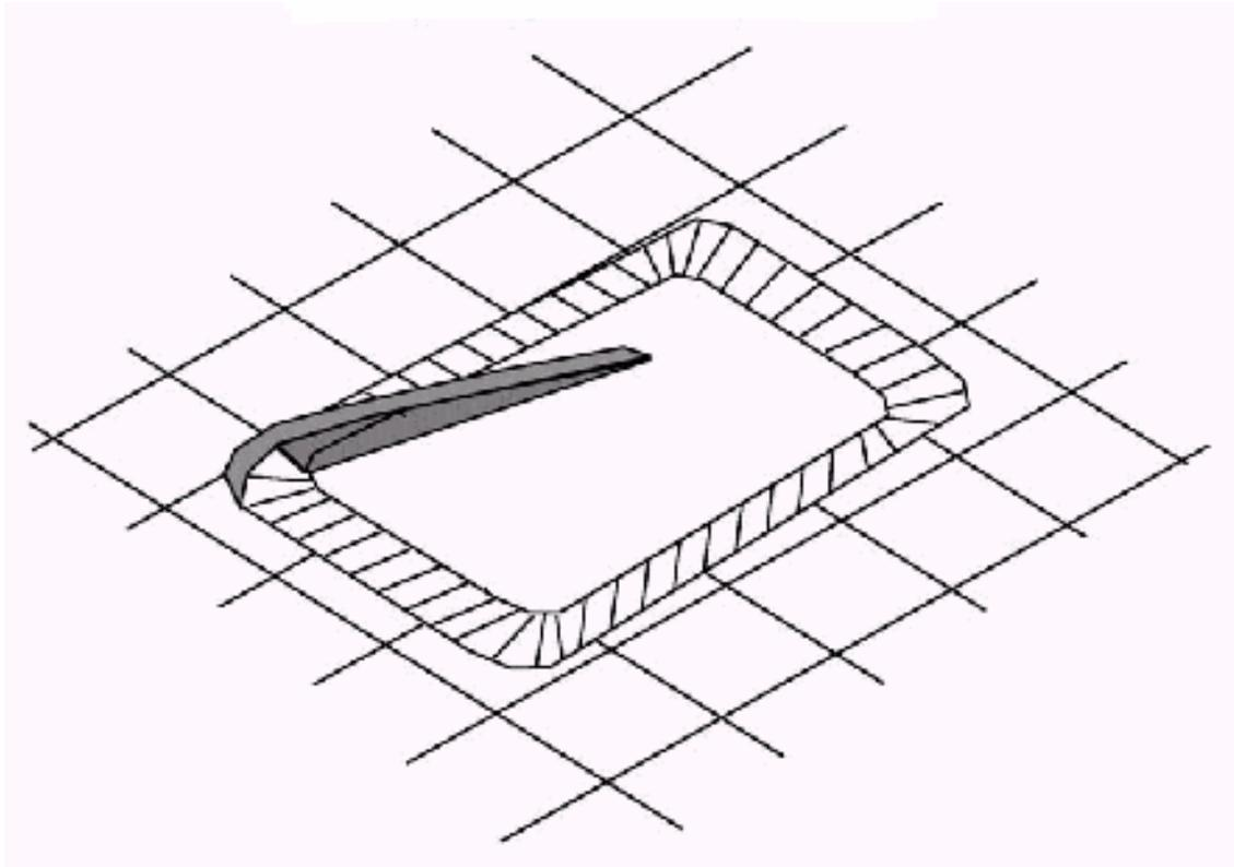
Figure 5. Geometry of a typical access ramp to a cell in a sanitary landfill (EPA, 2000)
