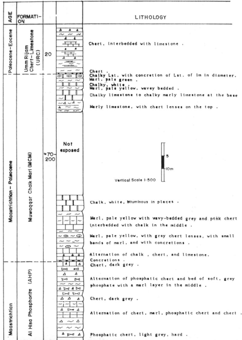
Figure 4. A geological column representing the formation at Ghabawi landfill
