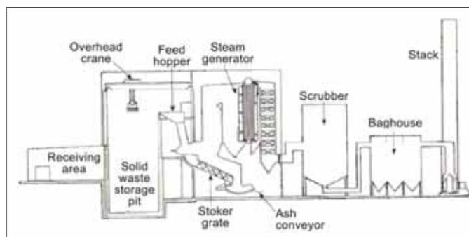
Fig. 2: Planned layout of the Santiago, Chile WTE plant. [24]
