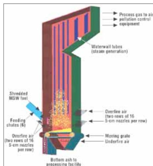
Fig. 3: Example of an RDF type facility, like the SEMASS facility in Rochester, Massachusetts, USA, which has a capacity of 0.9-million tons annually [Themelis, 2003].
