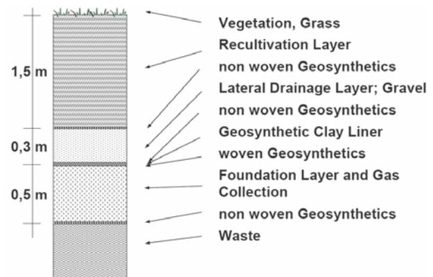
**Figure 3:** Different liner systems at landfill Zerbst (see also figure 4)
