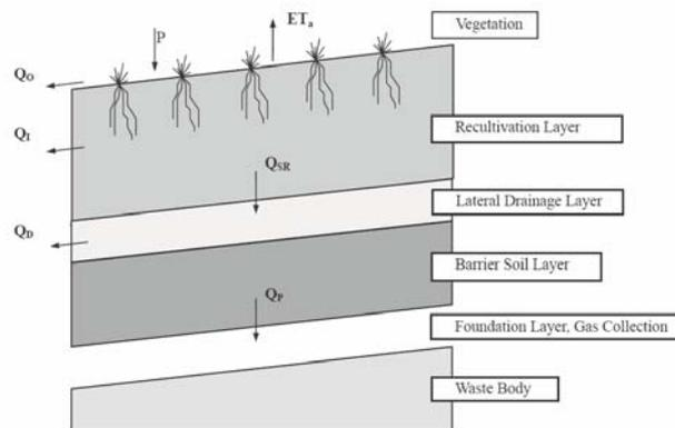
**Figure 2.** Schematic of a capping system profile (after BERGER, 2002)
