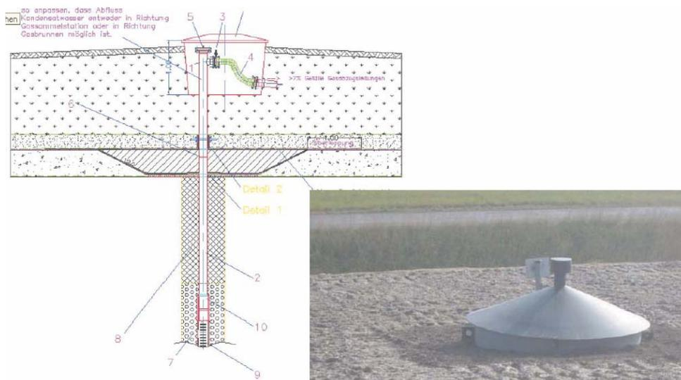
**Figure 8:** vertically gas collection system (head of gas well)
