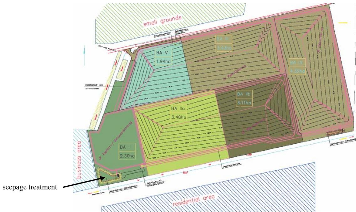
**Figure 4:** Position plan of landfill Zerbst, building sections and location in the city
