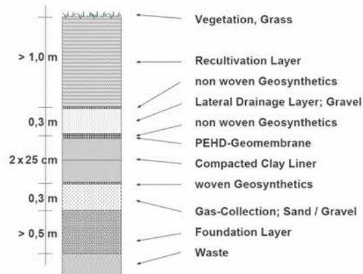
**Figure 1.** Capping system after TASI (1993)
