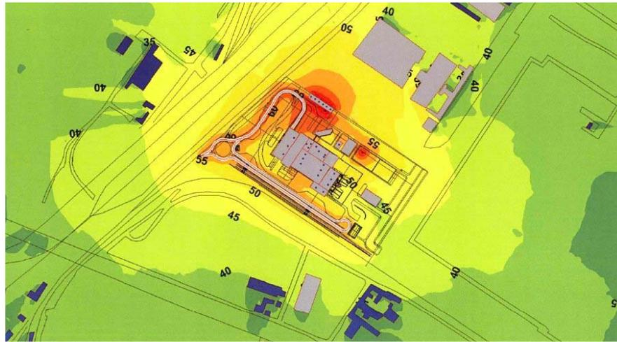
Figure 2. Noise generation: isophonic lines by day (data in dB(A)).
