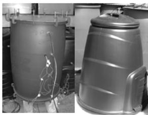
Figure 1. Forced aeration sealed compost unit (left) and naturally aerated open bottomed compost unit (right)
