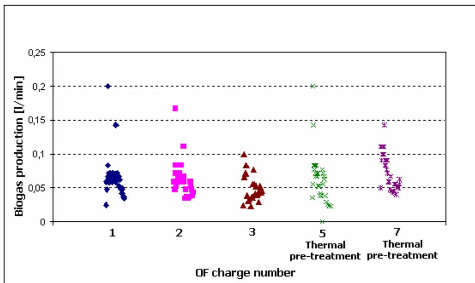
Figure 5. Comparison of biogas production after few hours later than OF feeding, in the case of absence/presence of thermal pre-treatment.
