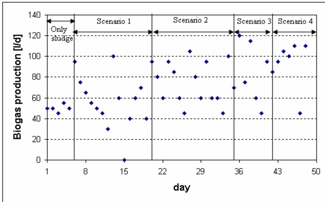
Figure 3. Biogas production during the experiments.
