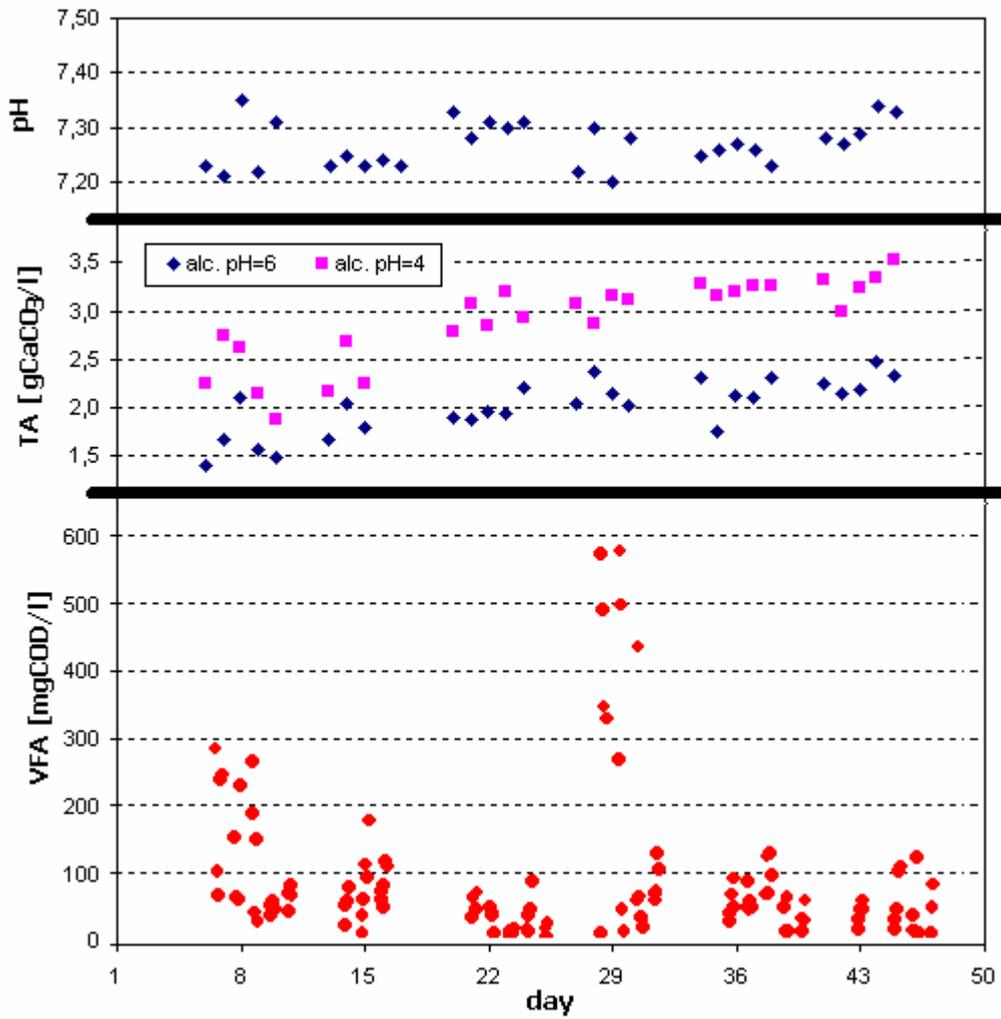
Figure 4. Trend of pH, Total Alkalinity and Volatile Fatty Acids during the experiments.
