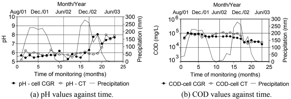
Figure 6. Leachate pH and COD values versus time in the experimental cells.
