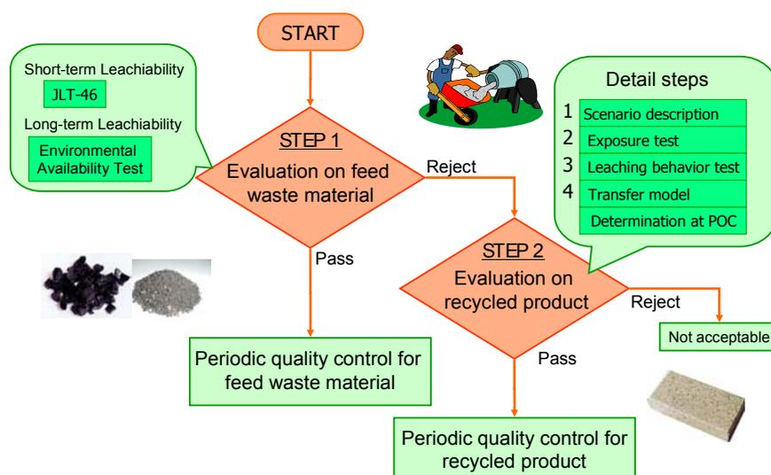
Figure 1. Evaluation frame for utilization of recycled products
