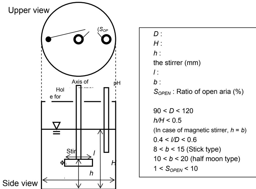
Figure 5. Test equipments for environmental availability test
