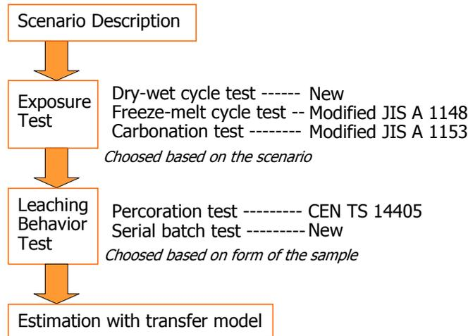
Figure 2. Adaptation of exposure test and leaching behavior test
