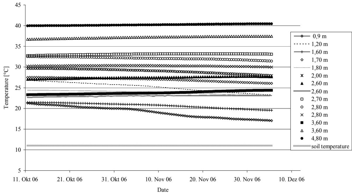
Figure 1. Temperature development in the MBW landfill body
