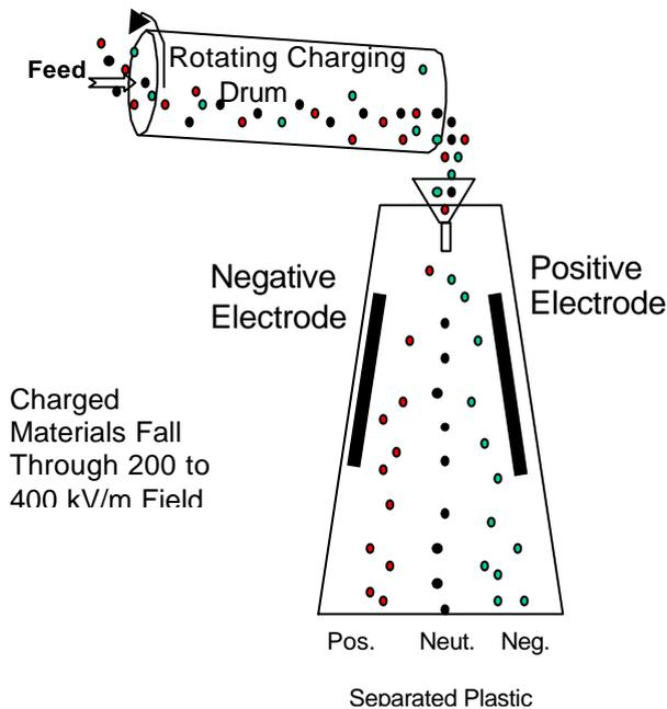
**Figure 2. Photo of Separation Unit**
