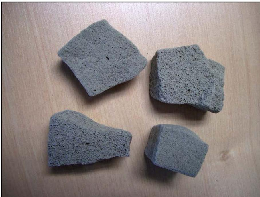
Figure. 4 Loose aggregate foam glass manufactured by Hasopor, Norway.
