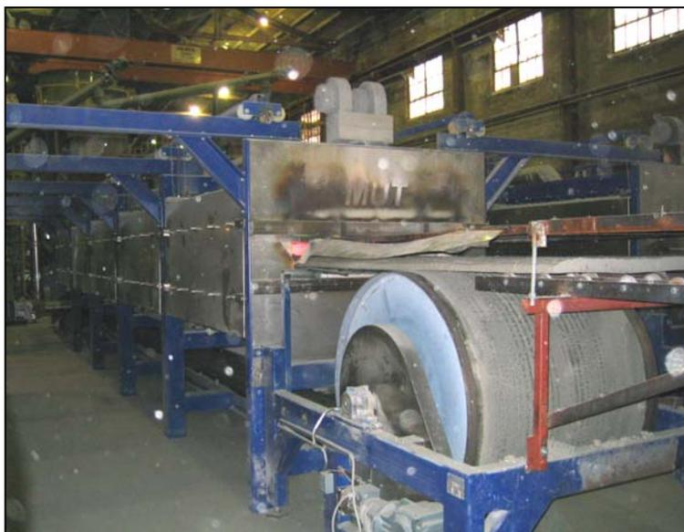
Figure 3. Foam glass merging from the furnace at Hasopor, Norway.
