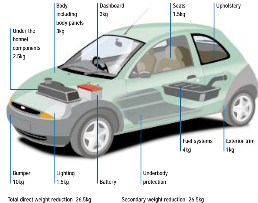
Substituting conventional materials with plastics leads to a direct primary weight reduction. The figures show the typical weight savings that can be made in various car parts. These then have a secondary effect as chassis, drive train and transmission parts can all be made lighter as a result.
