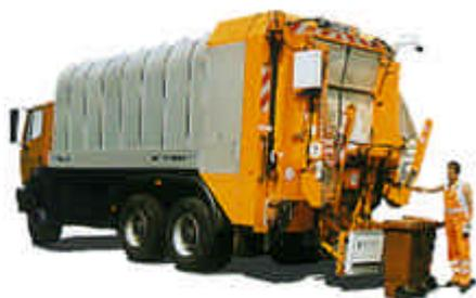
**Packer trucks** (revolving-drum or compression-plate vehicles) are standard for the collection of biowaste at the doorstep. Revolving-drum vehicles have the advantage that the compost material is thoroughly mixed during collection which is advantageous for subsequent decomposition and for a smaller amount of odorous leachate in the vehicle.
