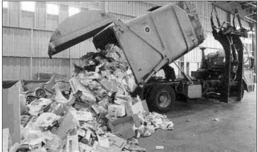
A collection vehicle dumps its load onto the tipping floor.
