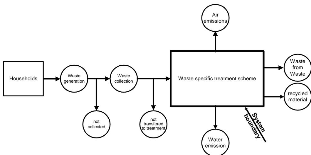
**The second step** is to define the unit operations within the system boundaries. This means that a specific treatment scheme is designed for each of the selected appliances. The unit operations are technical processes such as dismantling, shredding or metallurgical treatment. A system can be very simple e.g. in the case of disposal technologies it is limited to a single process. In the case of recycling the system can be complex and may comprise several unit processes.
