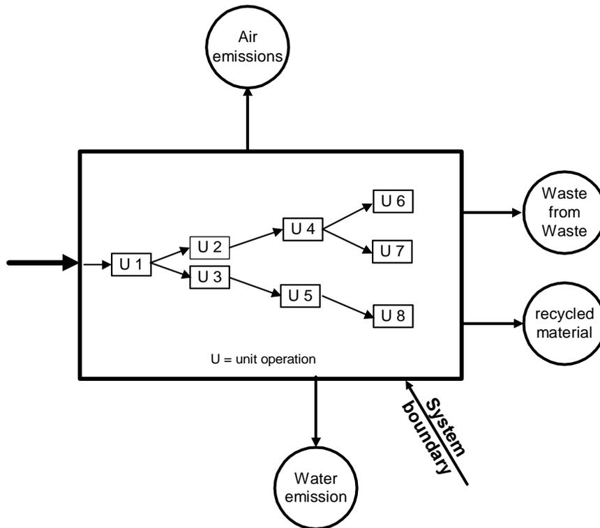
**The third step** is to describe the transfer of the substances in the various unit operations. This is done by assigning transfer factors for each substance and each unit operation. They are defined as follows:
