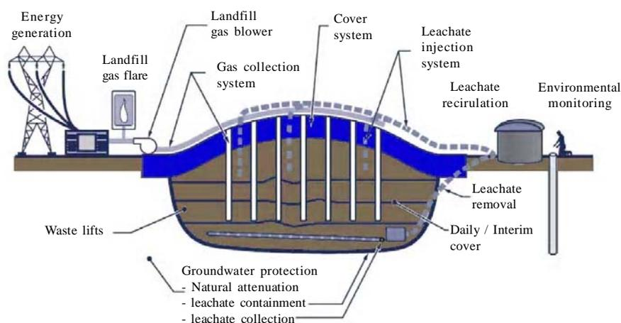
Fig. 1: Principal technical elements of a landfill ([FCM, 2004](#))
