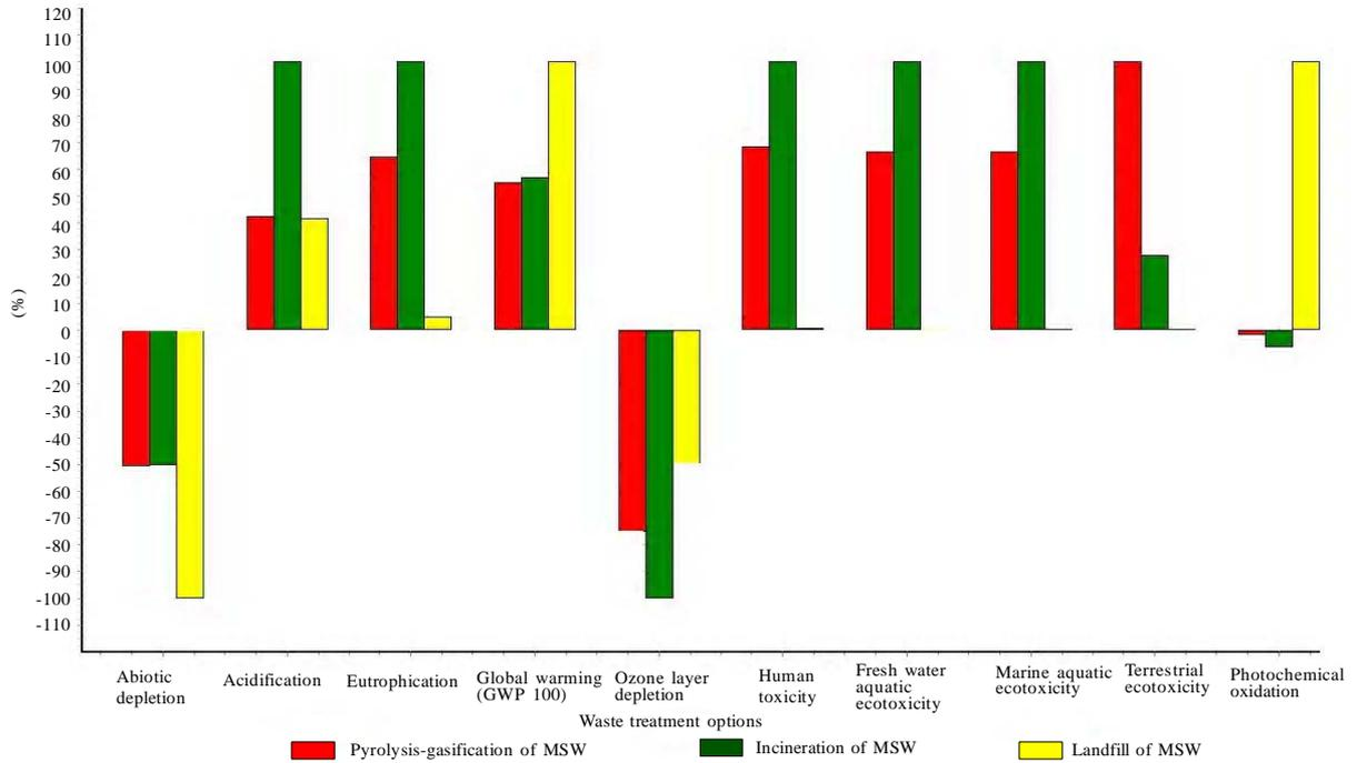
Comparing 1E3 kg 'Pyrolysis-gasification of MSW', 1E3 kg 'Incineration of MSW' and 1E3 'Landfill of MSW'; Method: CML 2baseline 2000 V2.04 / World, 1990 / characterization
