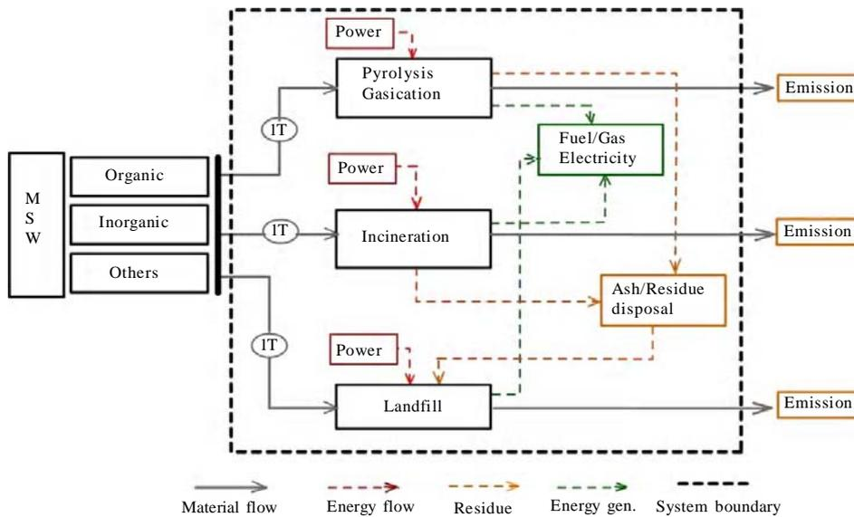
Fig. 4: System boundary for different MSW treatment processes
